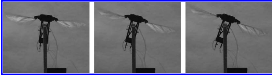
Fig. 20 MAV yawing as a result of asymmetric wing flapping amplitude modulation.
